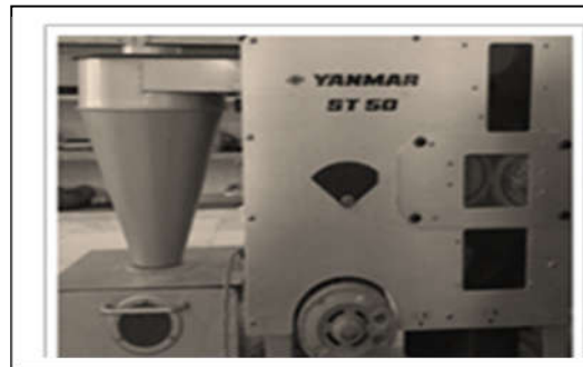
Fig (B) The machine (type Yanmar) which is used for hulling paddy
