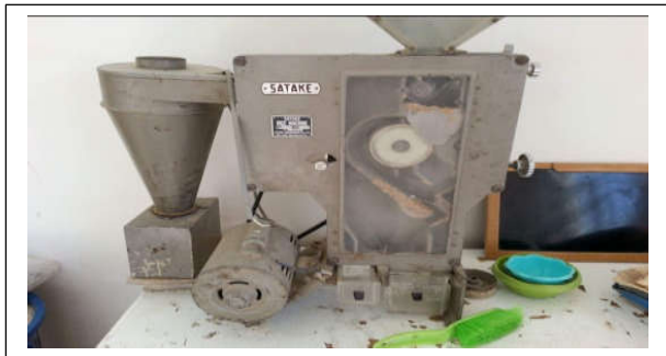
Fig (A) The machine (type Satake) which is used for hulling paddy
