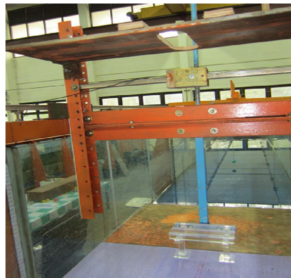
Figure 10. Photo of the bridge model installed inside the flume.
