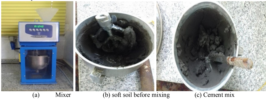
Figure 1: Preparing of the specimen in laboratory.
