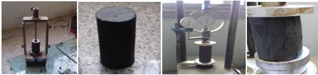
(a) Trimming Saw (b) Sample before Test (c) Sample during Test (d) Sample after Test Figure 3: Sample Trimming Saw, Samples before, during, and after Test.
