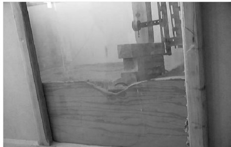
Fig. 10a: Failure mode for model footing without strengthening.
