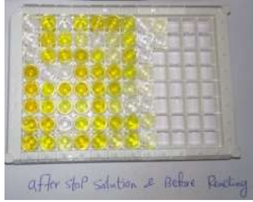
Photo (3): After adding 50 µl of the Stop reagent in order to stop the reaction & before reading
