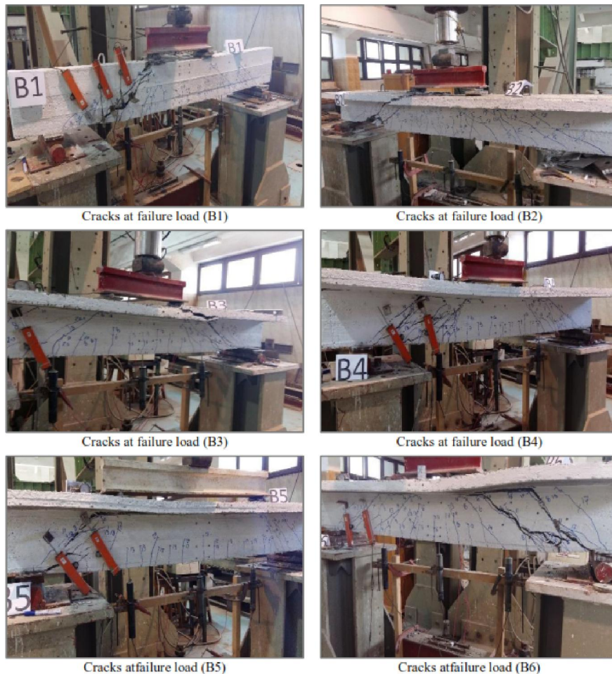
Figure 4: Crack patterns in the beams.
