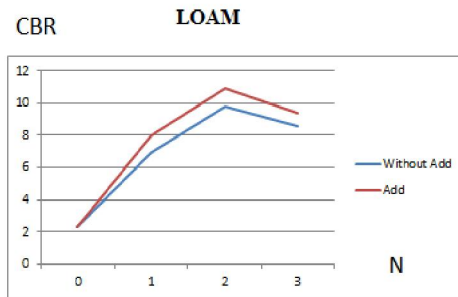
Figure (12): Effect of GEO1 at depths (1.5- 3- 4.5) cm in original and permazyme modified loam on (CBR) test.
