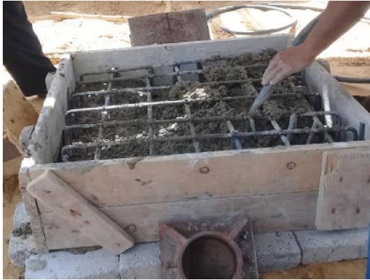
Fig (15) Shuttering, reinforcement and concrete casting for Piled-raft cap directly in contact with soil Group (2).
