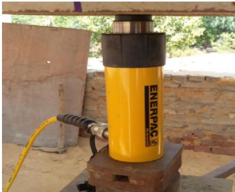
Fig (8) Loading jack and pump
