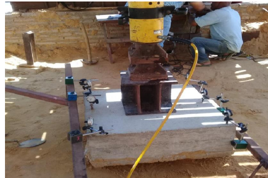
Fig (17) Loading jack, reference beams and dial gauges setup for Piled-raft cap freestanding Group (3).
