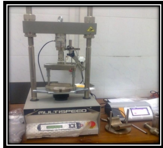
Figure (3) Indirect Tensile Strength Test Set-Up
