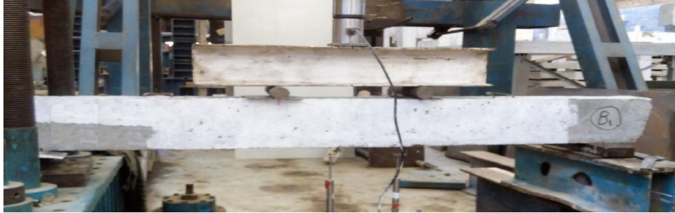
Fig. (4). 2-point beam tests of tested Beams by jack Capacity 200KN
