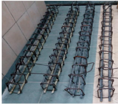
Fig. (1). Reinforcement details of Beams tested
