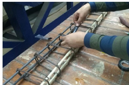
Fig. (3). strain gauge was mounting in mid span of the bottom bar to measure its strain
