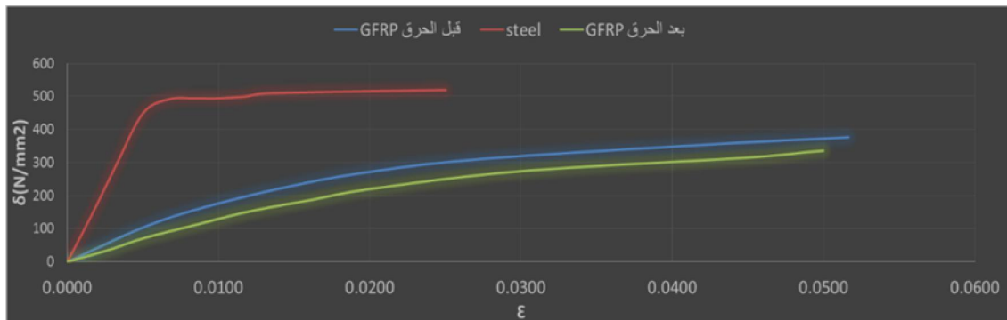
Fig. (10). Stress-Strain of GFRP bar before and after burning 400C and Steel bars
