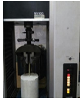
Fig. (15). Pull-out test for C.GFRP
