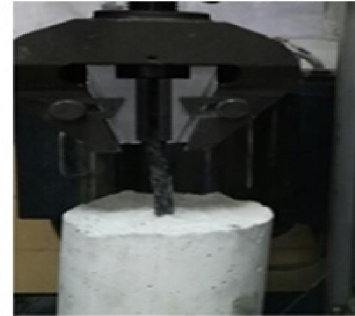
Fig. (15). Pull-out test for C.GFRP
