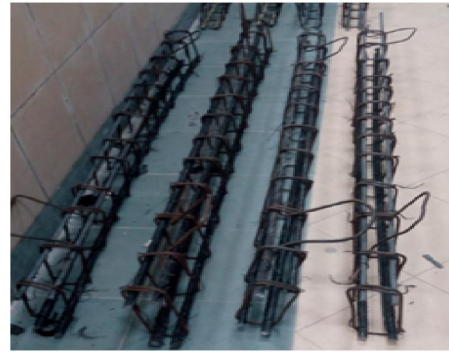
Fig. (1). Reinforcement details of Beams tested
