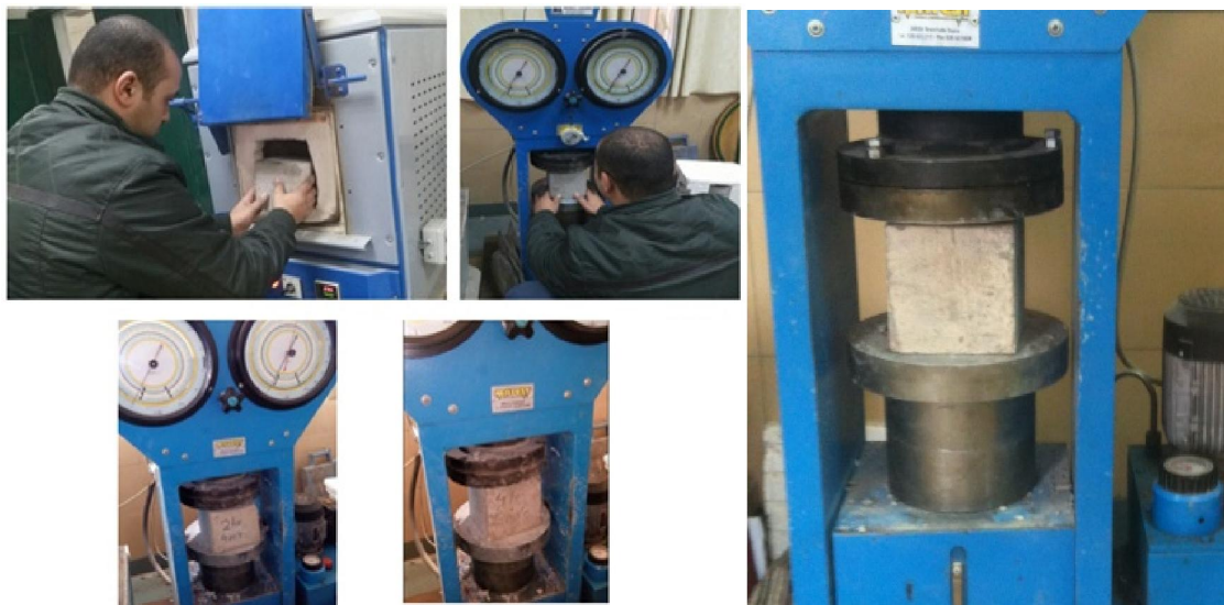
Fig. (18). Burning cube for 400°C and Compressive strength testing machine
