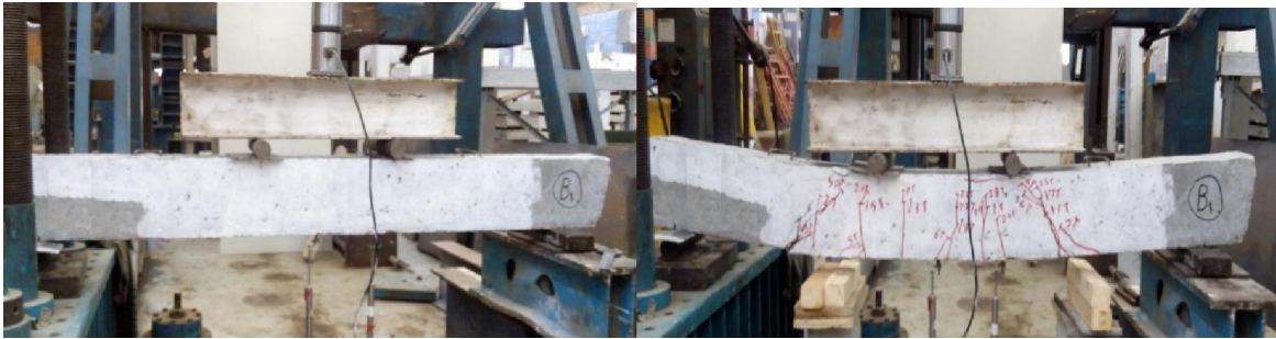
Fig. (19). Shape and values of cracks of (B1)
