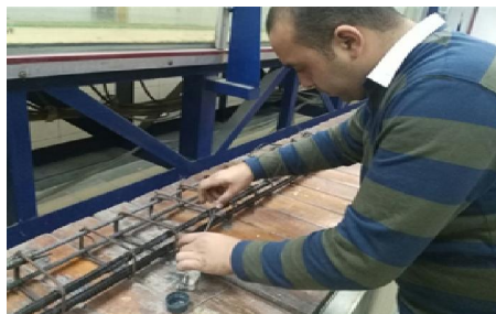
Fig. (3). strain gauge was mounting in mid span of the bottom bar to measure its strain
