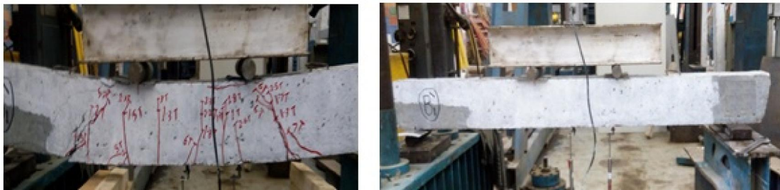
Fig. (20). Crack pattern of (B1) after burning at 400°C for 2 hours
