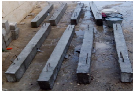
Fig. (2). Beam specimens casted before the beam test
