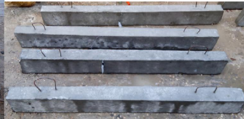
Fig. (2). Beam specimens casted before the beam test
