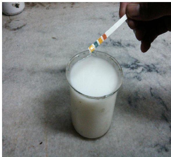
Figure 2.1(a): A PH strip is immersed in Resin
