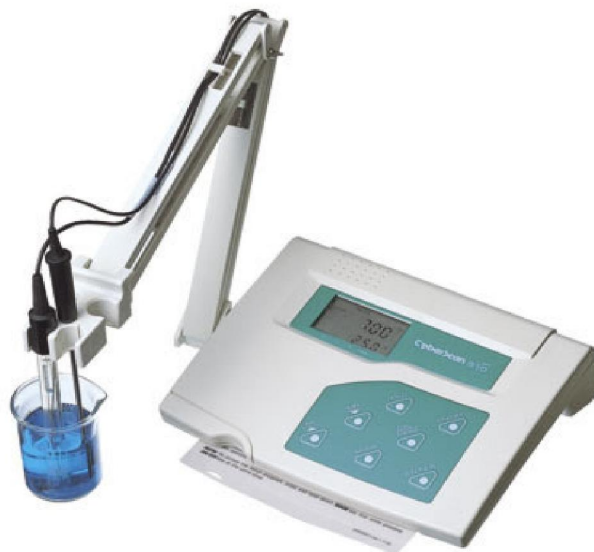
Figure 2.1(b): Digital PH Meter
