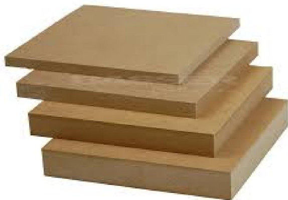
Figure 2.6: MDF pieces for Swelling in Thickness
