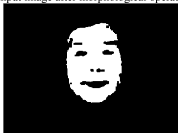
(b) Result after the 4-connected component labeling.
