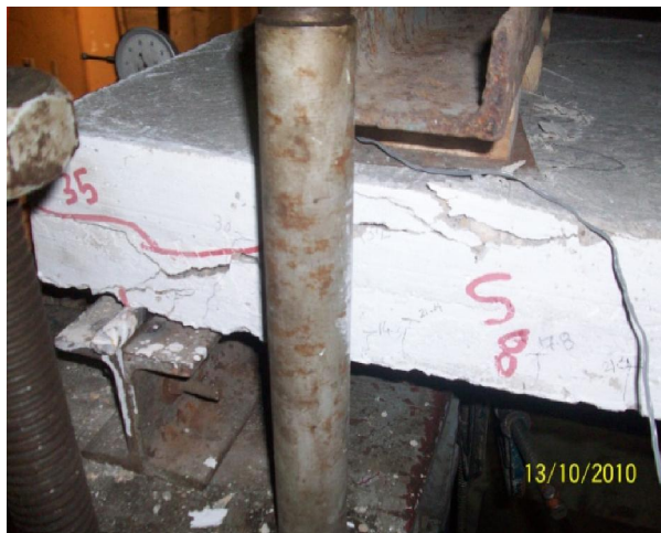
Figure (11): Shear failure of pre-slab S8.
