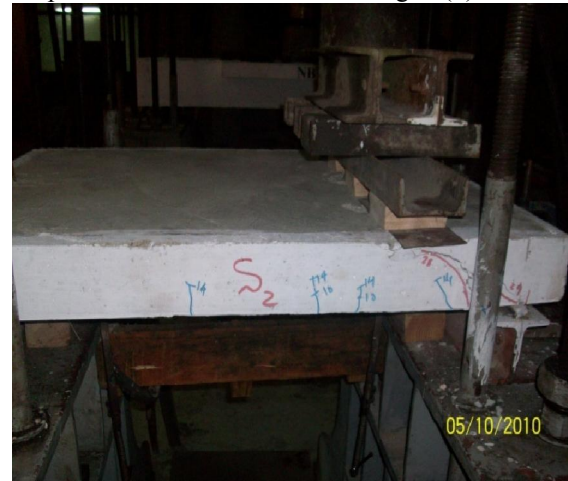
Figure (5): Shear failure of slab S2
